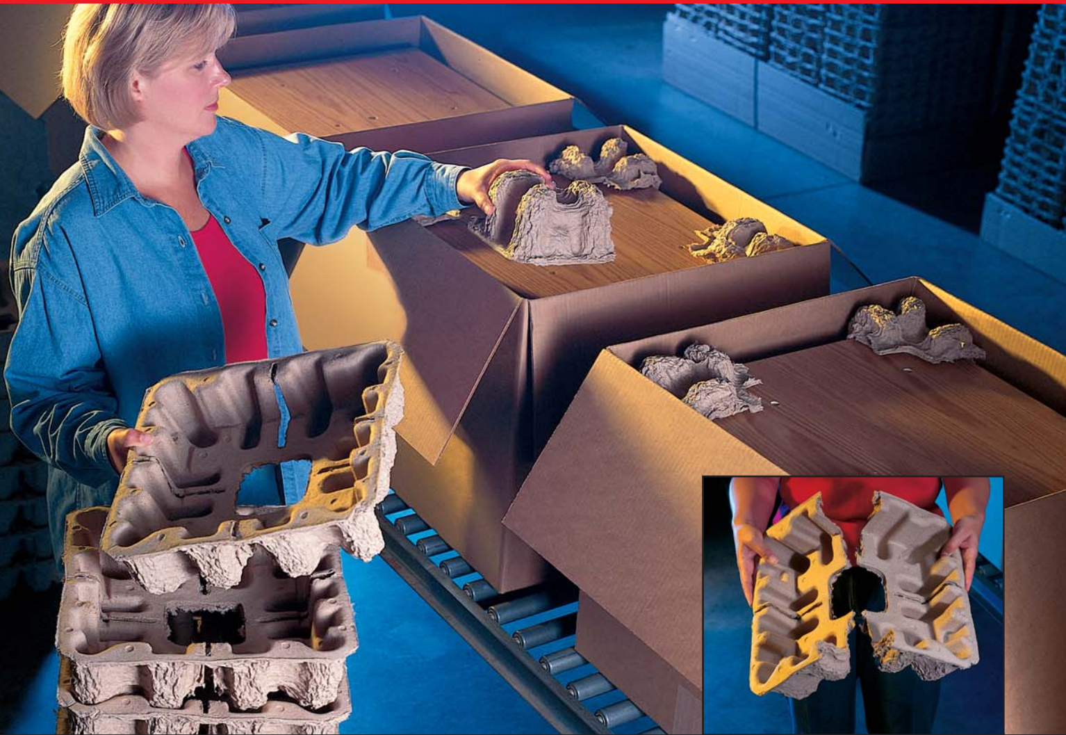
Break apart design improves packing line efficiency by reducing reaching motions.
